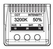
Press and hold right encoder for 1 second, invoking first set of presets. Immediately press and hold right encoder again to invoke second set of presets.
