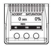
Press and hold left encoder for 1 second, invoking first set of presets. Immediately press and hold left encoder again to invoke second set of presets.
