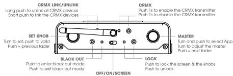
Select «screen off» position to turn off the display and save battery DMX data is still sent to the equipment
